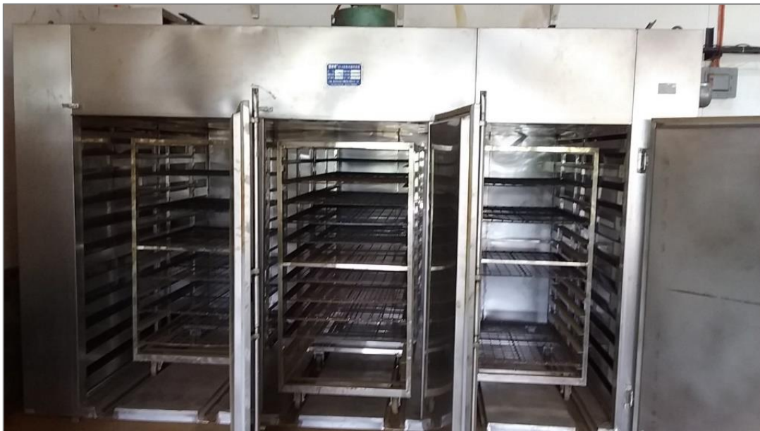
Figure 10-12. Electric oven for sample drying.
