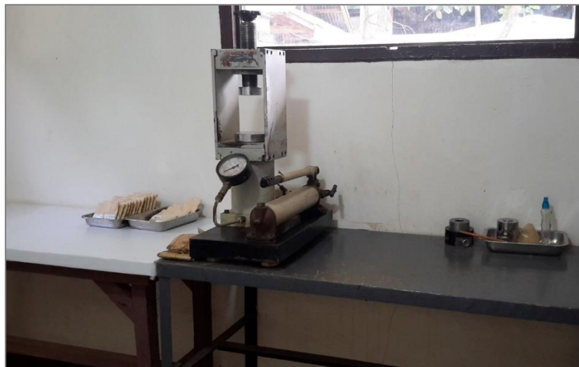
Figure 10-15. Hydraulic press for sample pelletizing.
