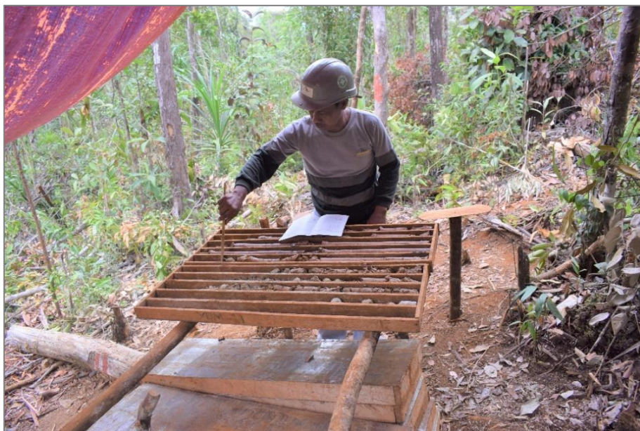
Figure 10-9. Core checking and logging at field camp.
