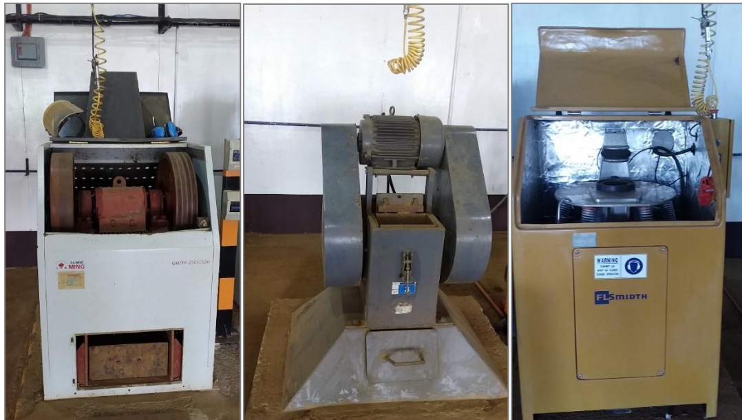
Figure 10-13. Primary jaw crusher, secondary jaw crusher and pulverizer.
