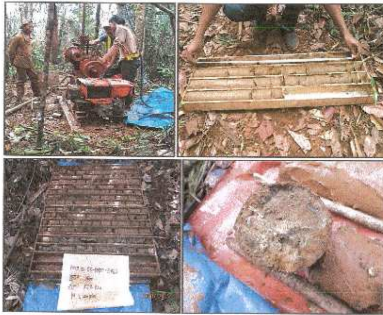
Figure 5-2. a) JGSI fabricated Koken drill machine, b) core samples placed in core boxes by the core checker, c) sample of core photograph taken once samples of a drill hole is delivered to the field sample house, d) sample of saprolite ore intercepted in one of the drill holes.
