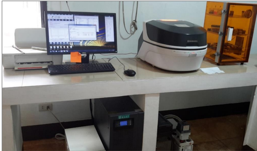
Figure 10-16. XRF-EDS Shimadzu brand with computer unit.
