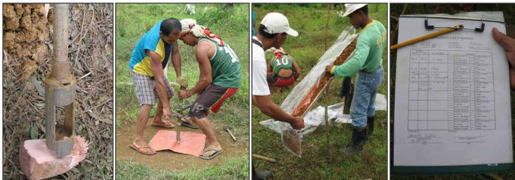
Figure 5-1. a) simple 20-centimeter long auger bit used by CNMC in its auger drilling activities, b) drillers retrieving the auger rods, c) samplers bagging the 2-meter composite sample, d) sample CNMC Checker's Daily Report.
